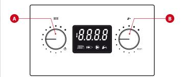
A. Setting the heating temperature and Summer/winter function: Range adjustable from 20 °C to 90 °C. When the thermostat is positioned on ∜, the heating circuit
